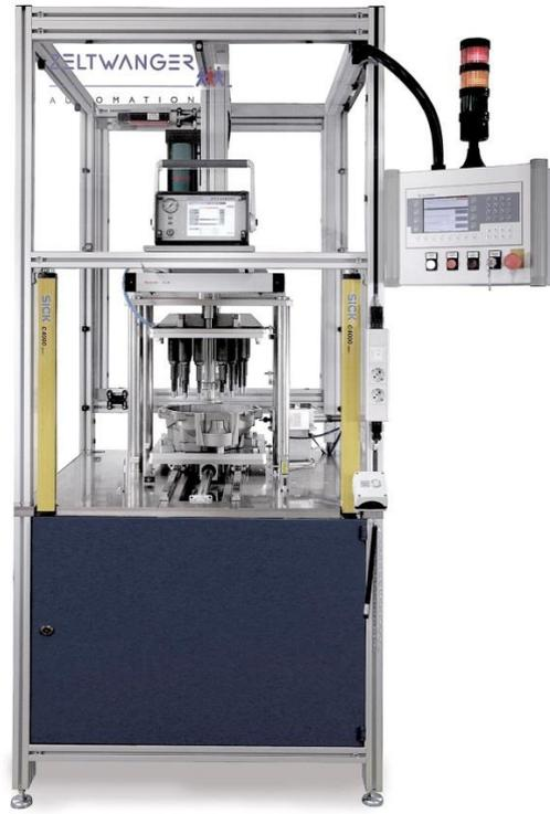
Image 2 shows the single carriage system including the mount for the gearbox casings (bottom) and the holding-down system (top), which presses the gearbox casing onto the sealing surface with a press force of max. 38.5 kN via TOX®-Powerpackage Drive Cylinders
